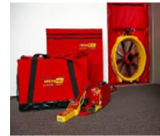
AIR TIGHTNESS TEST (HIGH PRES- SURE BLOWER DOOR SYSTEM) Measure amounts of Air Leakage.
